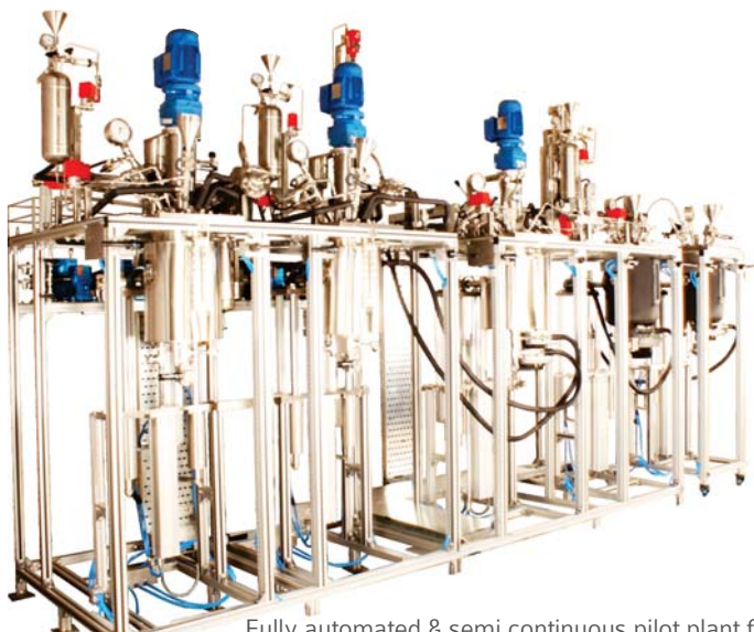
Fully automated & semi continuous pilot plant for styrene butadiene emulsion polymerization with pneumatic vessel raising, lowering & tilting
