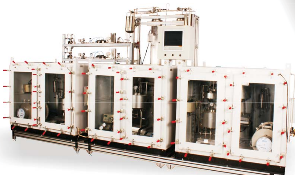
Pilot scale tubular reactor with purge panels for continuous biojet fuel production
