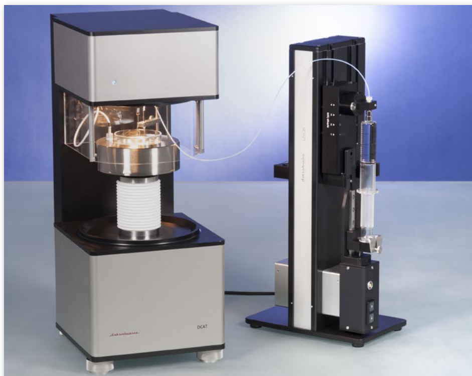
Determination of the critical micelle concentration with a DCAT 15 and LDU 25 with a syringe holder SH-LDU
