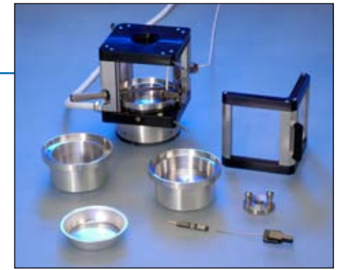
TEC 250/DCAT – electrical temperature control unit with accessories
