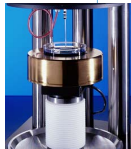
TV 70NM – non-magnetic thermal chamber with removable micro-electronic stirrer
